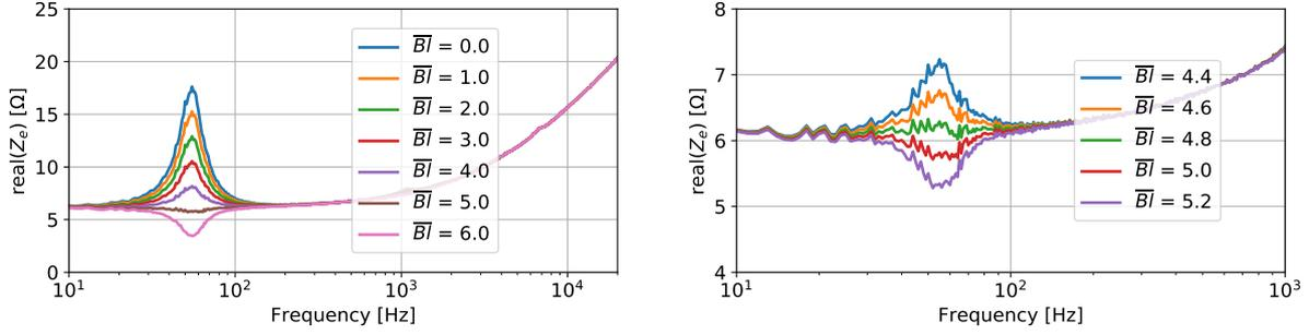
Figure 4. Graphical representation of the force factor  $Bl$  estimation from the measured data. The value of  $\overline{Bl}$  that removes the resonance from the electric impedance  $Z_e(\omega)$  is selected as the best estimate of  $Bl$ .
