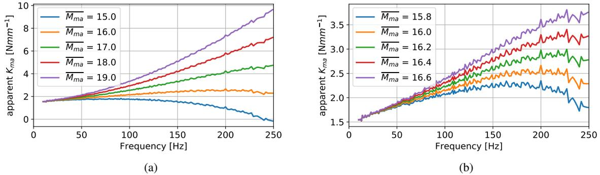
Figure 8. Estimation of the apparent stiffness  $K_{ma}(\omega)$  and the mass  $M_{ma}$  from the measured data.
