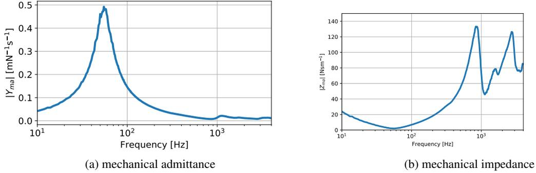
Figure 6. The absolute value of the mechanical admittance (a) and the mechanical impedance (b) as a function of frequency, estimated from the measured data.
