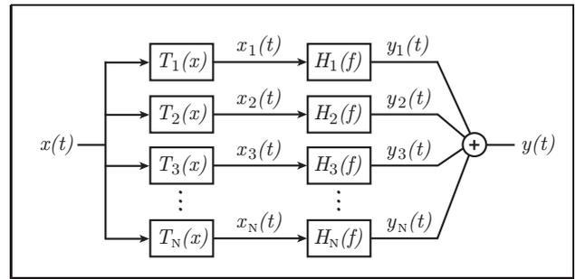
Figure 1. Nonlinear woofer model with Chebyshev polynomials  $T_n(x)$  and higher order frequency responses  $H_n(f)$ ,  $x(t)$  is the input signal,  $y(t)$  the output signal and  $n$  the order taking the values from 1 to  $N$ .
