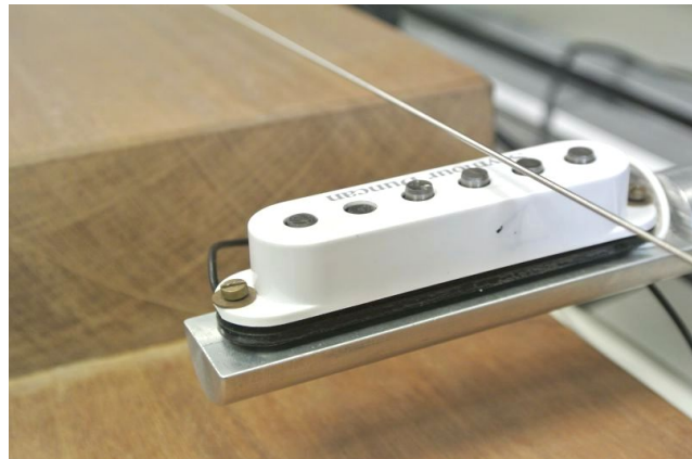
Figure 9: Picture of the second experiment in which the pickup is placed under a vibrating string.
